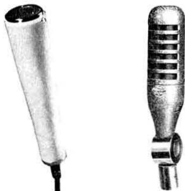
The Acos Mic-39-1 microphone (left) and the Lustraphone VR.64. Both are suitable for stereophonic recording.
